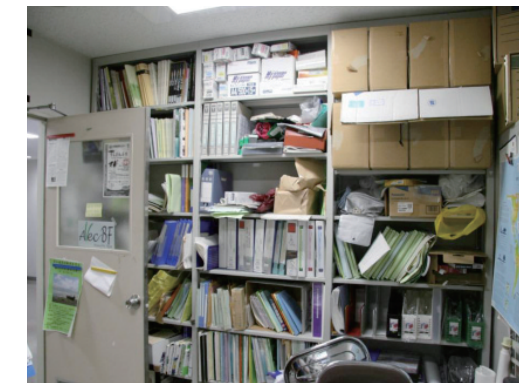
Shelves which will block the aisle when they fall (in Nagoya Univ.)
